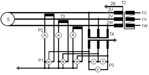
picture 7: test setup for measurement of excitation
