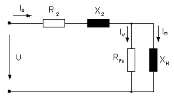
picture 6: transformer in no-load
