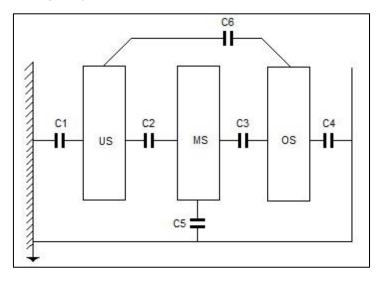
picture 10: test setup for capacity measurement at three-winding transformers
