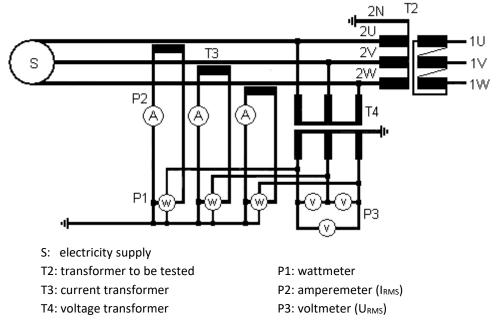
picture 3: test setup for measurement of sound level
