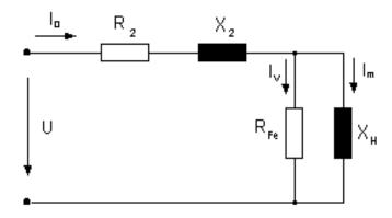
picture 2: transformer in no-load
