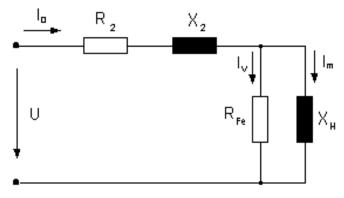
picture 20 transformer in no-load
