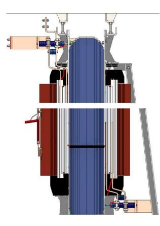
picture 11: transformer active-part cross-section
