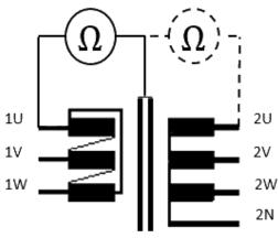
picture 14: test setup for insulation resistance
