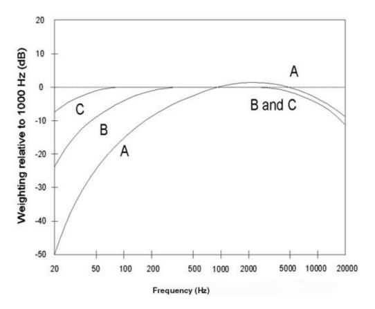
picture 1: sound level meter response characteristics for the A, B, and C weighting
