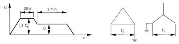
picture 22: measurement of partial discharge with earth
