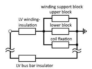
Therfore it could happen that e.g. the isolator of the LV busbar (if existing) creates a parallel circuit (picture 13: equivalent circuit diagram of the main insulation parts) with winding support and LV insulation. In this case the winding support and the winding insulation (with e.g. cast resin) could be irrelevant (depending on conditions).
